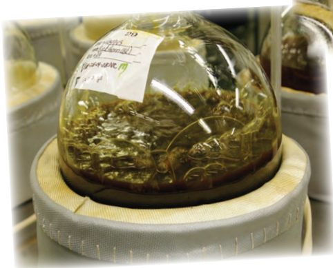
Blackthorn in its seventh day of the water extraction step. Bubbles occur spontaneously when precipitants break the liquid's surface tension in the beaker.
